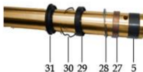
(31) CACHE POUSSIÈRE (30) CLIP (29) JOINT SPY (28) RONDELLE (27) BAGUE FIXE (5) BAGUE COULISSANTE
